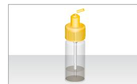
Break off the tip of the screw cap of the tube.
