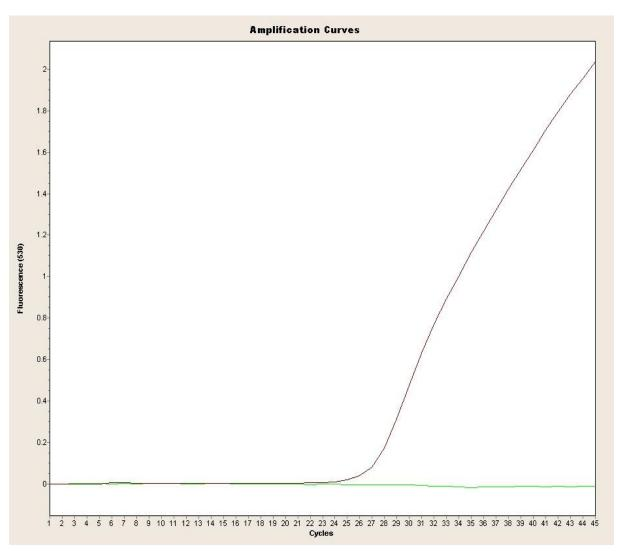
Fig.1: Correct run of the positive and negative control (SCCmec / orfX junction) on the LightCycler<sup>®</sup> 2.0
