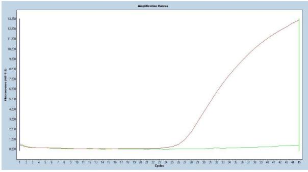
Fig. 1: Correct run of the positive control (red) and negative control (green) (*Bacteroides*) on the LightCycler<sup>®</sup> 480II
