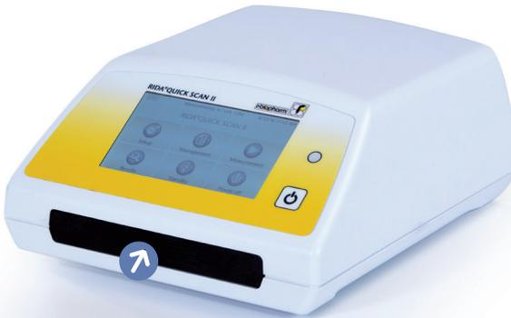
**Fig. 9:** Slightly press the front plate of the drawer to open it
