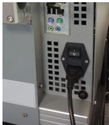
Figure 4: The mains lead attached to the power inlet socket of the instrument
