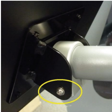
Figure 2: touchscreen rear clamp mounting
