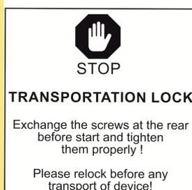
**Fig. 2.:** How to remove the transportation lock
