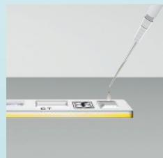
Place the test cassette on a flat level surface. Using the supplied microliter pipette, place 150 µl of the supernatant in the application area of the test cassette.
