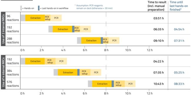
Depending on the workload RIDA®UNITY allows you to process up to 3 runs or up to 384 reactions in one day. Start processing the next samples while your PCR is still running.
