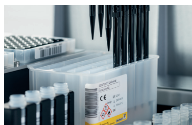
The extraction of up to 96 samples is processed fully automatically
